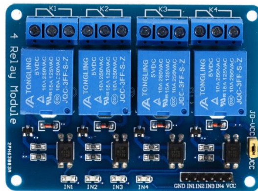
Figure 7 - 5 volt operated 4-channel relay module
