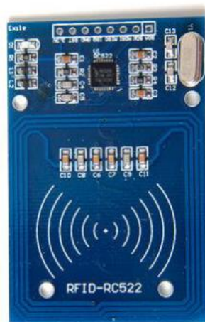
Figure 6 - RFID based security module
