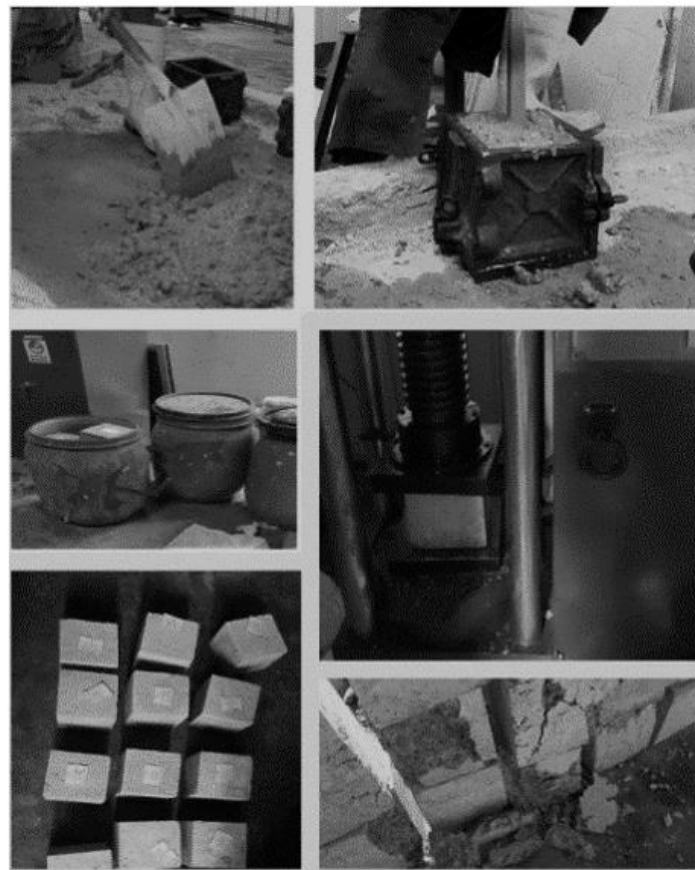
Figure 2: Test cube casting and testing process
