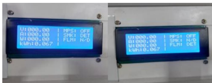
Figure 11 - Smoke Detection (SMK: DET) and Flame Detection (FLM DET)
